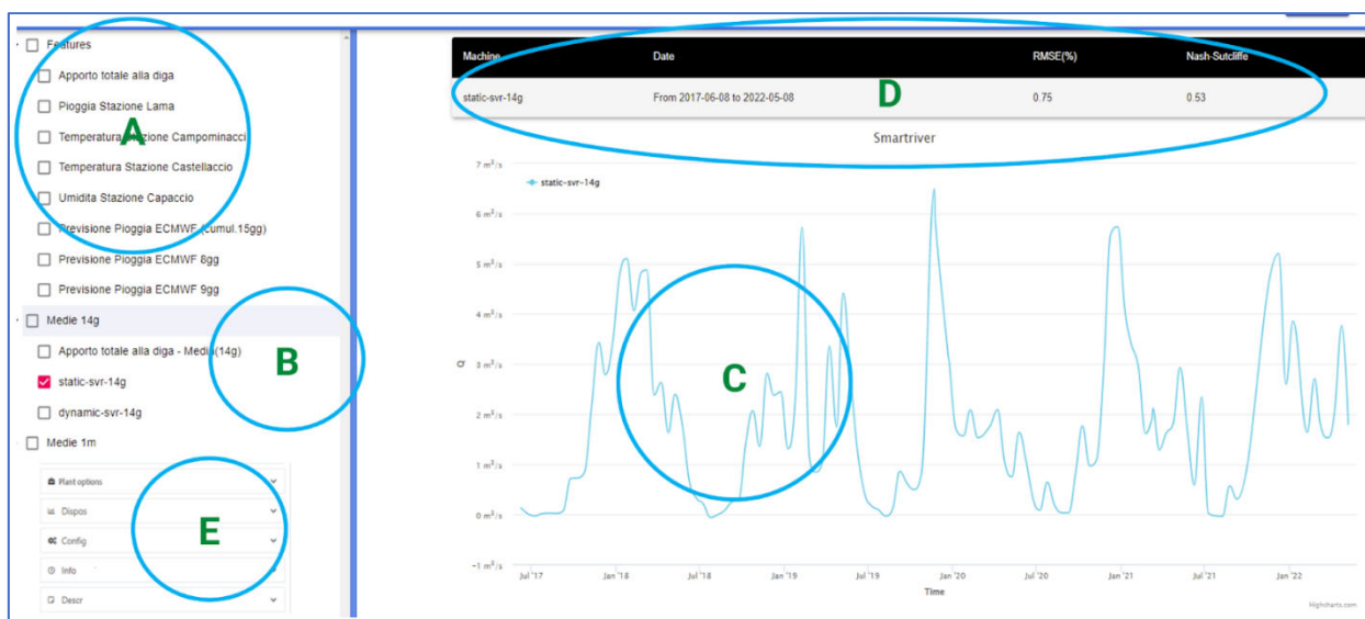
Figure 17 Sketch of a possible service GUI. A: Input features (e.g. rainfall and temperature, ground stations or averaged, recorded discharge, meteorological forecast); B: discharge forecast for lead times of interest; C: Time series of variables of interest; D: Lumped error metrics for the selected period; E: Configuration options; F: error graphs and graphic indicators of forecast performances (see also next figure).
